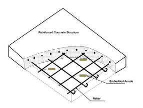
Reinforced Concrete Structure Installation Holes for Sacrificial Anodes
