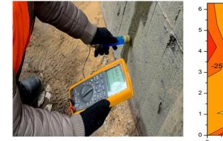
**ASTM, C876-09 (2009)**, Standard Test Method for Half-Cell Potentials of Uncoated Reinforcing Steel in Concrete (USA and international).
