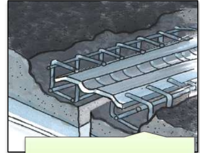
Road joints fastening
