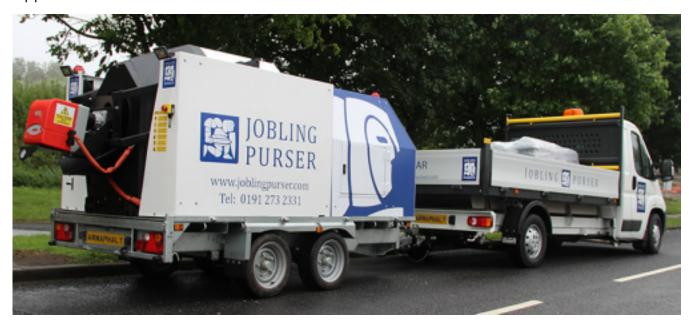
The Armaphalt is placed into the machine, heated and mixed as required.
