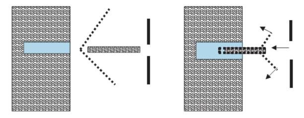
6. After the installation of the Ardfix® apply the required longitudinal reinforcement layers, as they have been determined by the study, in the side of the component / member, using epoxy resin Betontex ® RC or fireproof resin Betontex ® IPN. The final assembly is shown in pictures below.
