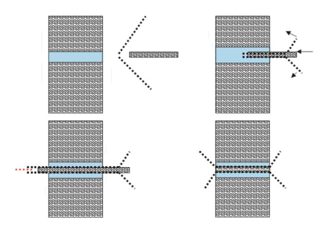
6. After the installation of the Ardfix® apply the required longitudinal reinforcement layers, as they have been determined by the study, in both sides of the component / member, using epoxy resin Betontex® RC or fireproof resin Betontex® IPN. The final assembly is shown in pictures below.
